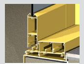
Standard tall, small, beveled and square rails are all an option. Standard tall splayed bottom rail illustrated above
